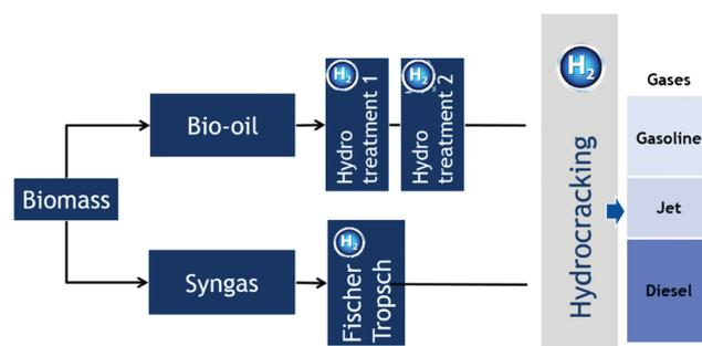
Figure 9. Simplified schematic of thermochemical conversion technologies.
