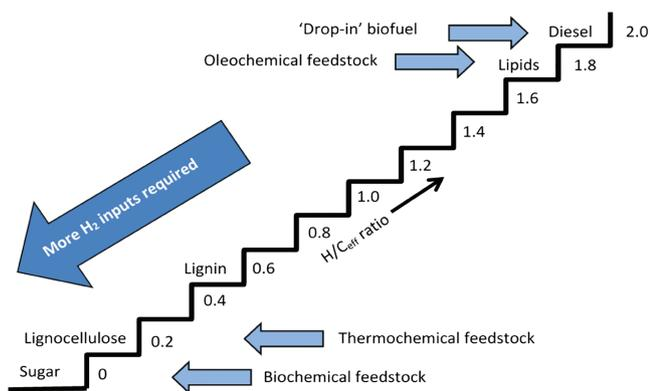
Figure 6. The effective Hydrogen to Carbon ratio 'staircase' for feedstocks.
