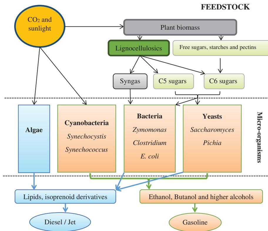
Figure 12. Schematic overview of the micro-organism-to-drop-in-intermediate or biofuel derived for various renewable feedstocks. Adapted from Weber et al.<sup>31</sup>
