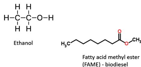
Figure 2. Chemical structure of ethanol and FAME biodiesel.
