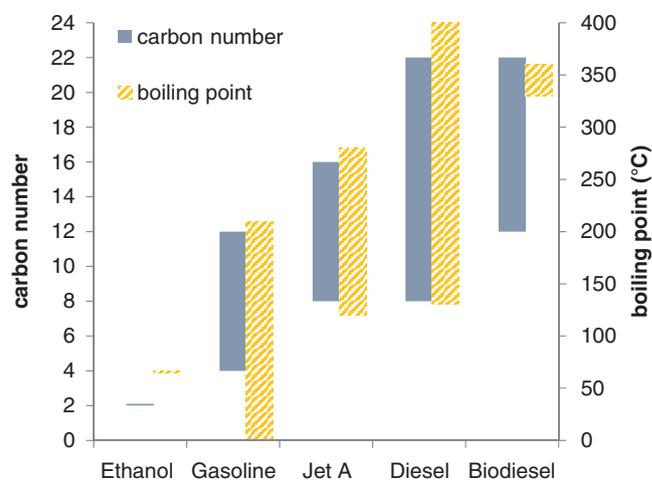
Figure 4. Carbon number and boiling point range of commercial transportation fuels.<sup>6</sup>
