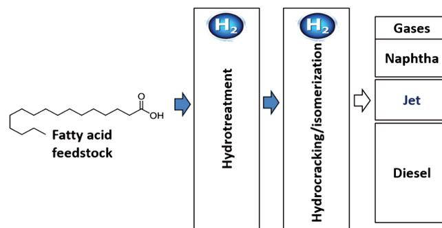
Figure 7. Simplified schematic of the oleochemical conversion process.
