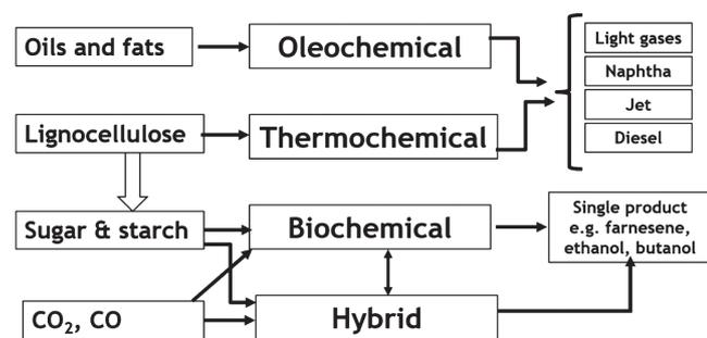
Figure 5. Simplified diagram of different technology routes to drop-in biofuels.
