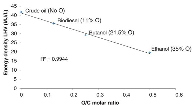
Figure 3. The effect of oxygen content on the energy density of liquid fuels.
