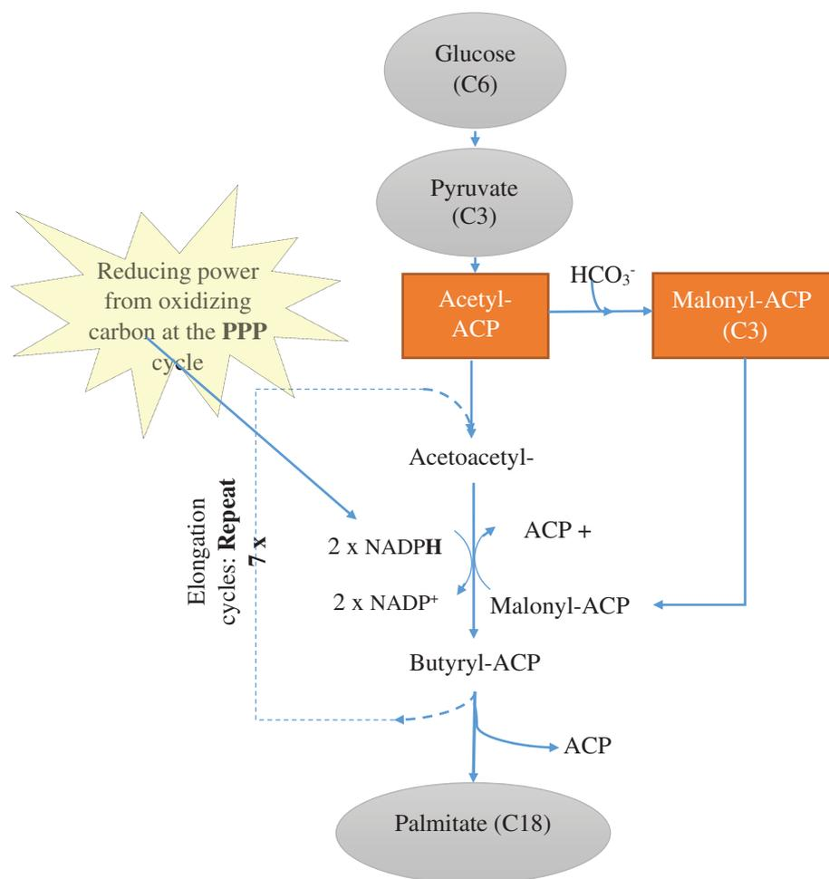
Figure 14. Biosynthesis of fatty acid, palmitate clearly illustrating the addition of hydrogen from NADPH. A total of 14 hydrogen atoms are required and this reducing power is acquired from oxidizing of carbon at the PPP. Adapted from Jovanovic Tews *et al.*<sup>24</sup>
